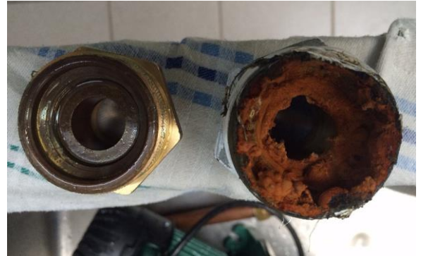
Left as it should be, right with legionella contamination (Maritiem Courant Jan 2020).
